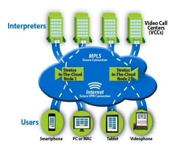
The Stratus video network platform is a fully redundant, dual core network interconnected with three different telecommunications carriers for Internet access, three carriers for telephone service (PSTN) access and 30+ video call distribution centers across the United States on a self-healing MPLS network. This network has given Stratus an extremely reliable service, with availability for the last three years exceeding 99.99%.
